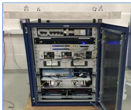
Figure 6. Open air spent fuel monitor installed at Fukushima Daiichi
